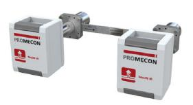
Until now, measuring the off-gas from electric arc furnaces involved intrusive sensors or extractive measurements in the exhaust gas channel, which only provided the measured values with a delay or required high maintenance. In contrast, the new McON IR sensors operate on an infrared basis and do not require lances protruding into the off-gas duct. They measure chemical composition as well as the velocity and temperature of the off-gas stream directly at the off-gas manifold.
